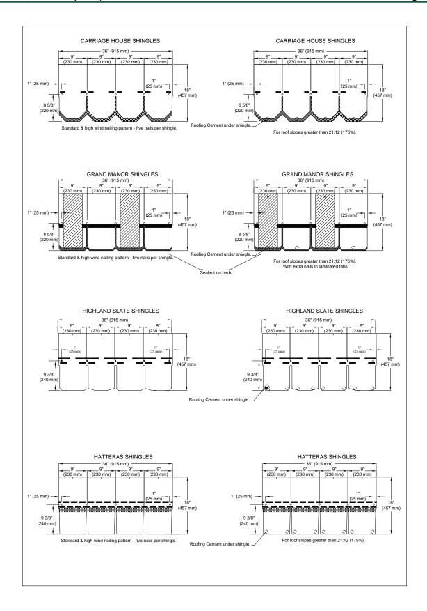
FIGURE 1—SHINGLE PROFILES AND FASTENER PATTERNS (Continued)
