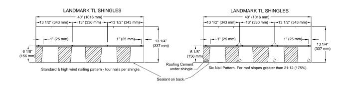
FIGURE 1—SHINGLE PROFILES AND FASTENER PATTERNS (Continued)
