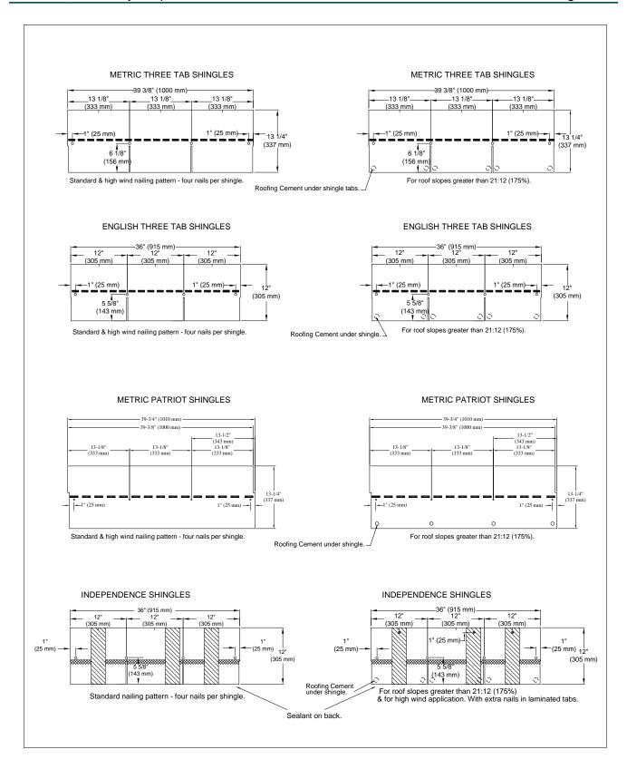
FIGURE 1—SHINGLE PROFILES AND FASTENER PATTERNS
