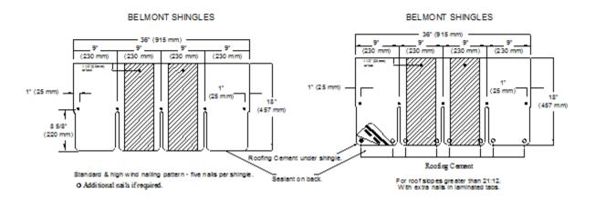
FIGURE 1—SHINGLE PROFILES AND FASTENER PATTERNS (Continued)
