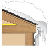
WinterGuard is installed under shingled roofing to prevent water damage from ice dams, as well as wind-driven rain.
