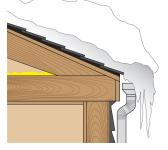
When snow and ice melt, trapped water can infiltrate to damage the roof deck and building interior.
