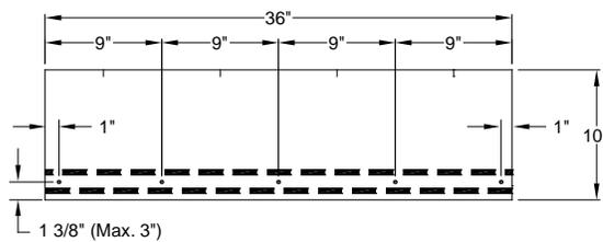
Standard nailing pattern for all slopes from 2/12 (16.7%) up to and exceeding 21/12 (175%) & for high wind application.
