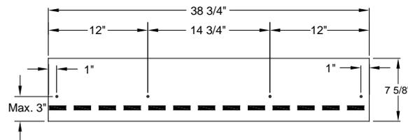
Standard nailing pattern for all slopes from 2/12 (16.7%) up to and exceeding 21/12 (175%) & for high wind application.
