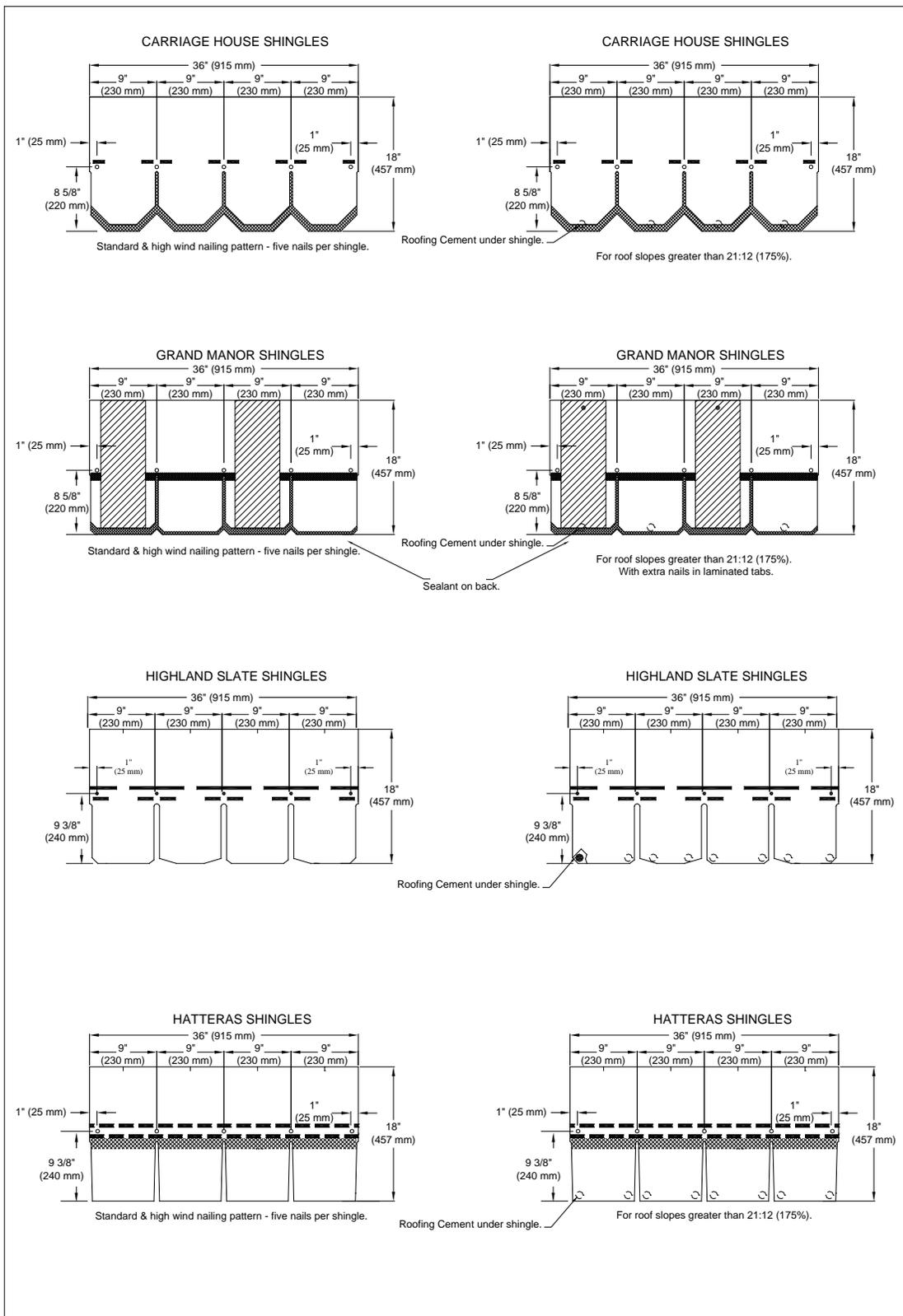
FIGURE 1—SHINGLE PROFILES AND FASTENER PATTERNS (Continued)
