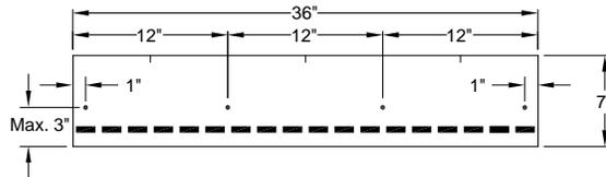
Standard nailing pattern for all slopes from 2/12 (16.7%) up to and exceeding 21/12 (175%) & for high wind application.
