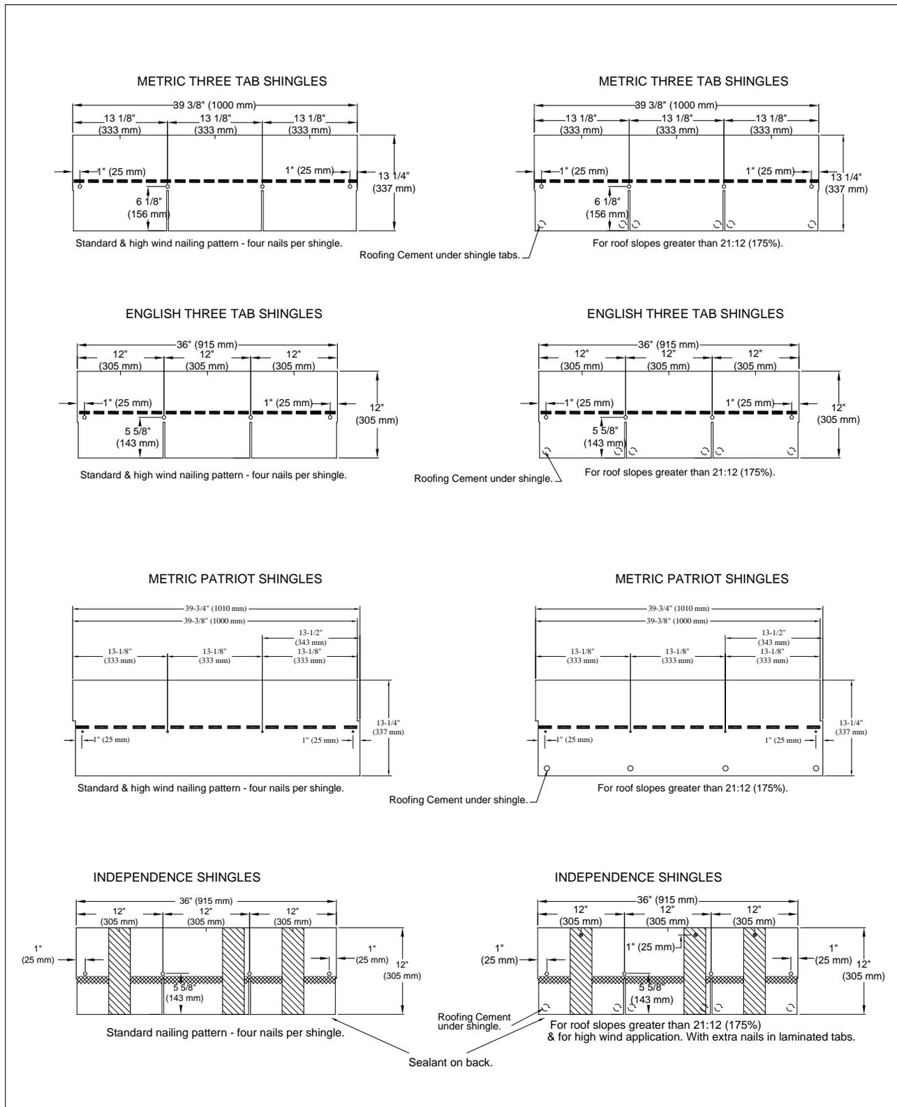
FIGURE 1—SHINGLE PROFILES AND FASTENER PATTERNS
