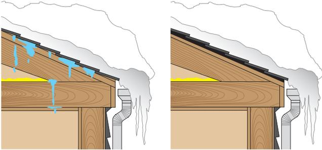
When snow and ice melt, trapped water can infiltrate to damage the roof deck and building interior.
