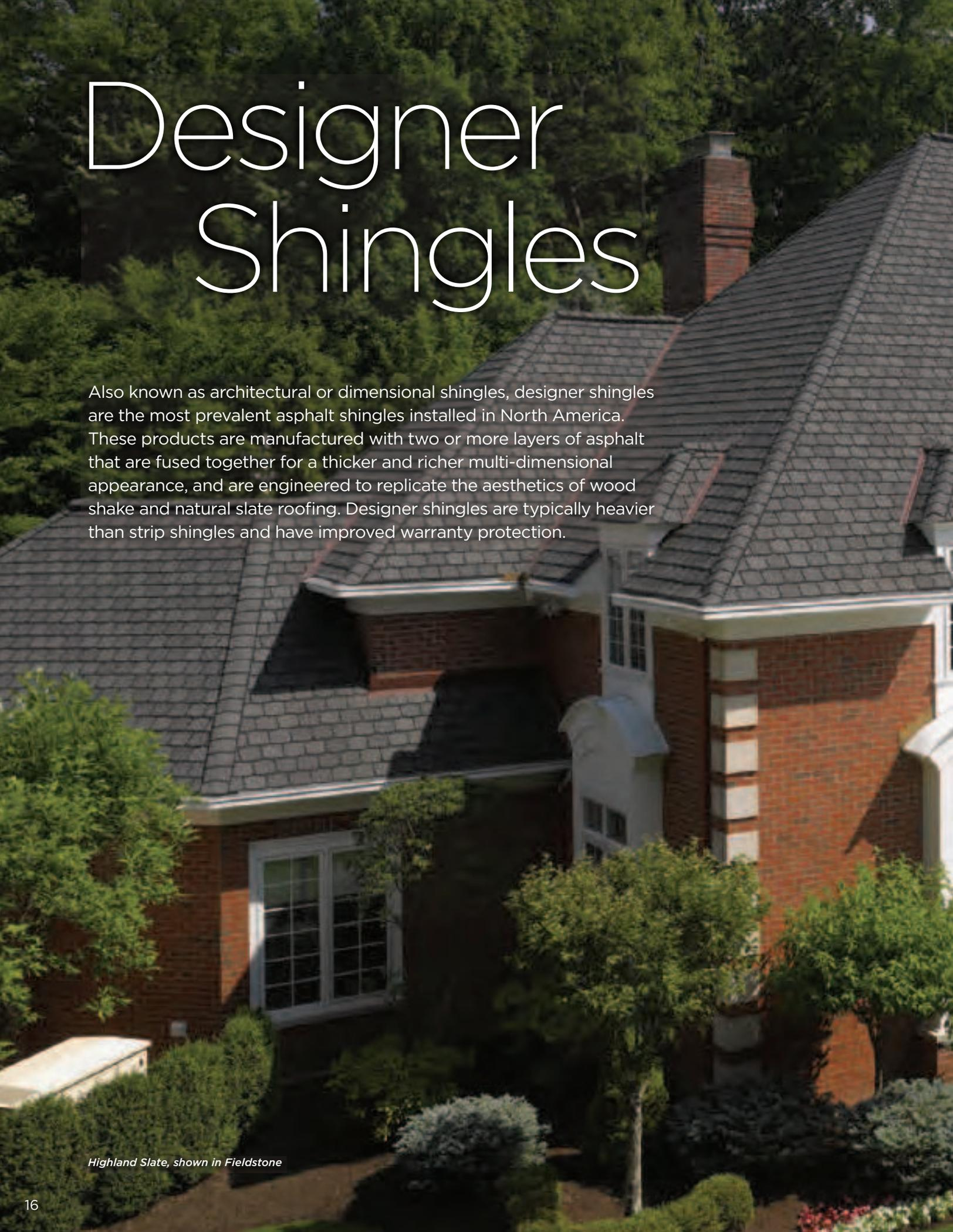
Also known as architectural or dimensional shingles, designer shingles are the most prevalent asphalt shingles installed in North America. These products are manufactured with two or more layers of asphalt that are fused together for a thicker and richer multi-dimensional appearance, and are engineered to replicate the aesthetics of wood shake and natural slate roofing. Designer shingles are typically heavier than strip shingles and have improved warranty protection.
